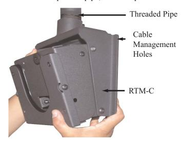
. Place the RTM-C coupler onto the threaded end of the suspension pole. Thread the coupler onto the threaded pipe tighten at least seven (7) complete turns.
